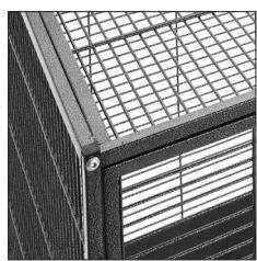
**EN** Slide the roof panel in the top grooves of the side panels. Fix now at the top all the top panels with screws.
