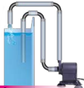
OPERATING OUT OF THE WATER WITH PIPES AND HOSES
